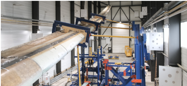
Biaxial test fatigue setup with spring element and decoupled masses
